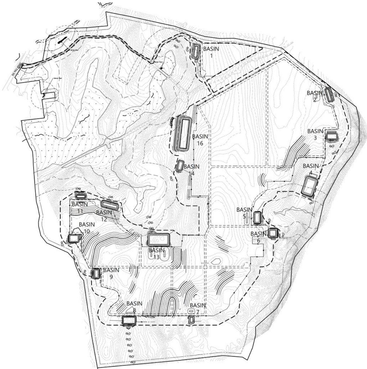
FIGURE 1. Stormwater detention basins located within the Waterford solar energy site.
